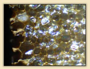
This is an image from the opposite face of the sample. Note the exact same result showing exposure of the initially damaged outside cells with **no** further penetration into the body of the sample.
