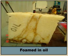
It is always preferable to remove as much contamination within the pontoons as possible. Minor residues of hydrocarbons are swept into the lower parts of the foam without ill effect. Very small amounts of water are acceptable however a layer of standing water may disrupt cell formation over a larger volume and should be removed.
